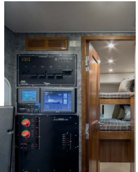
PowerPlex ® controls and monitors the entire on-board electrical system and always keeps the owner and crew up-to-date on the electrical systems via touch screens.
