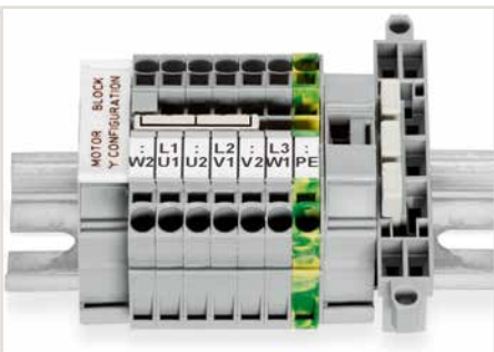
This star point jumper has been specially developed to create a "star point" and is used on motor terminal boards equipped with TOPJOB® S rail-mount terminal blocks.
